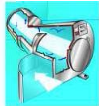
Hydrobrake in high storm event. Central vortex is created which displaces water to further control discharge rates.
